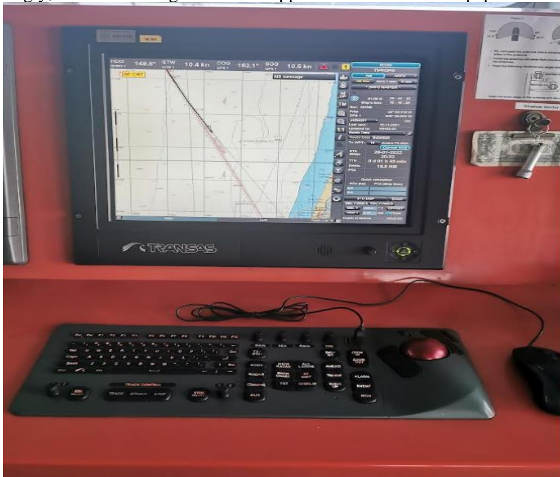
Figure 1 - Electronic navigational charts on the navigation bridge equipment
