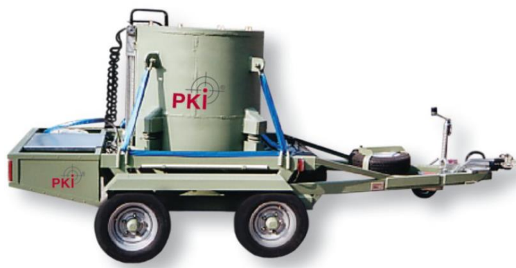
Fig. 3 – PKI 9275 Trailer system for transporting of explosive objects
