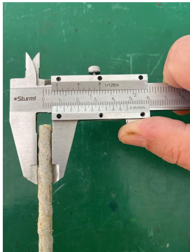
Figure 2. Samples of fiberglass reinforcement with sand coating under research.
