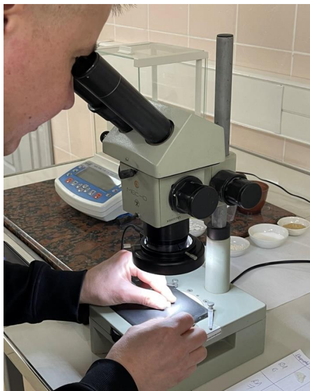
Figure 3. Microscopic examination of samples of fiberglass reinforcement.
