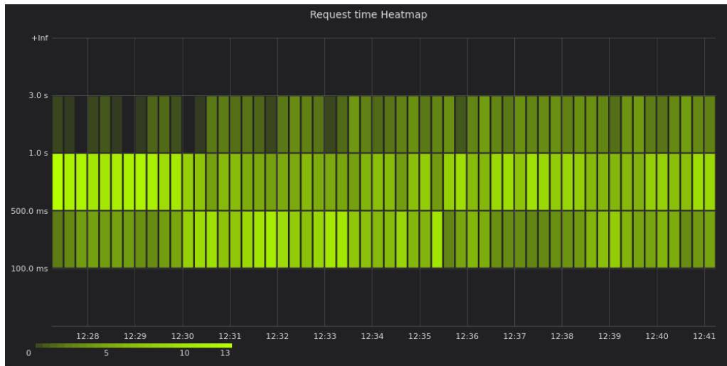
Figure 6. Heat maps with the distribution of query times in Accumulo for 50 users writing at the same time.
