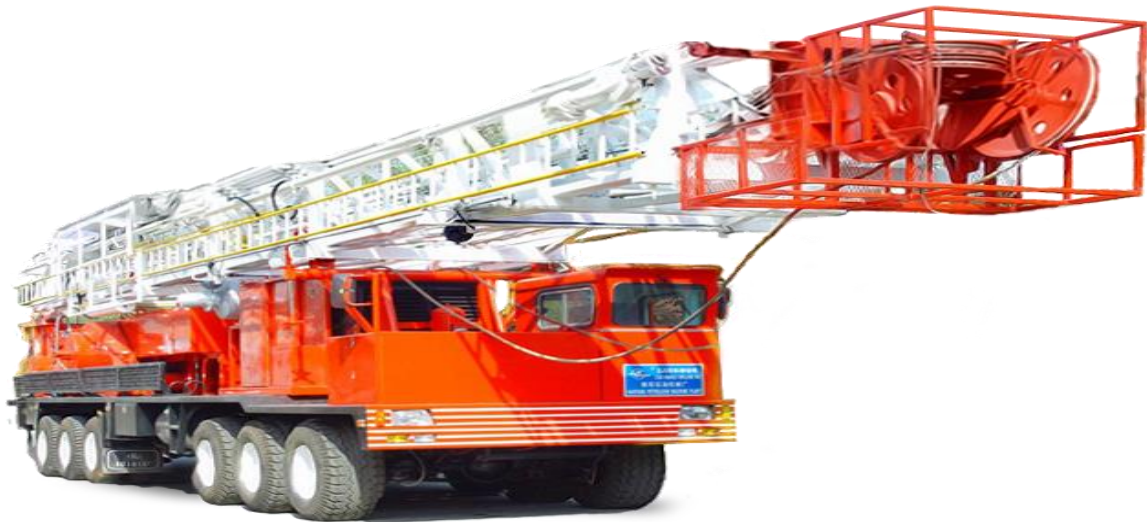
Figure 1. Mobile drilling installation XJ1000
