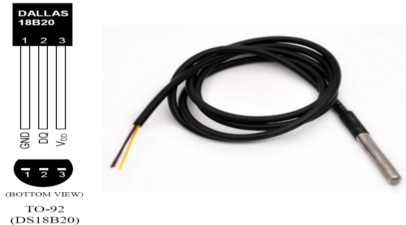
Figure 1. DS18B20 thermal sensor and its positioning within the casing.
