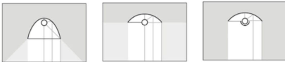
Figure 3. Radiation Flux Distribution Depending on Parabolic Reflector Design
