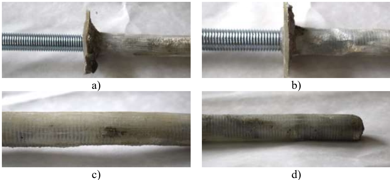
Figure 3. General views of the threaded rods extracted from cells P3V3 (a) and P4V3 (b). Detailed views of the embedded sections of the rods from P3V3 (c) and P4V3 (d), demonstrating full and uniform coverage of the threads with epoxy resin. Source of the figures: author's archive.
