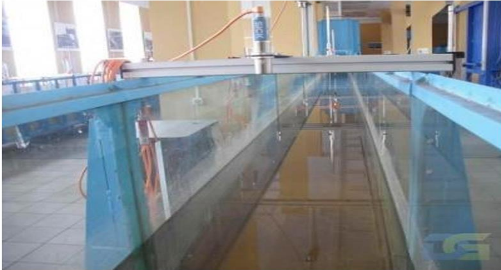
Figure 2. General view of the wave flume used for investigating the effects of wind-generated waves. [Developed by the author].
