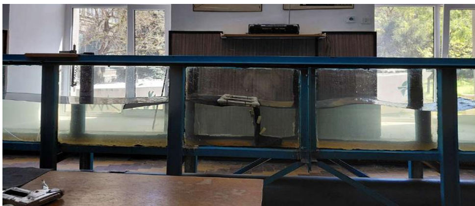
Figure 4. Methodological experiments on investigating the wave attenuation efficiency of the flexible breakwater model (Model 2). [Developed by the author].
