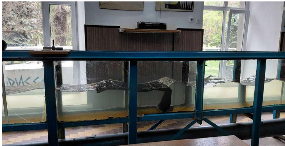
Figure 3. Methodological experiments on investigating the wave attenuation efficiency of the flexible breakwater model (Model 1). [Developed by the author].
